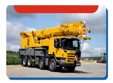
The truck crane is a simple lifting engineering vehicle, which is mainly used for lifting and transporting cargo of small tonnage.
